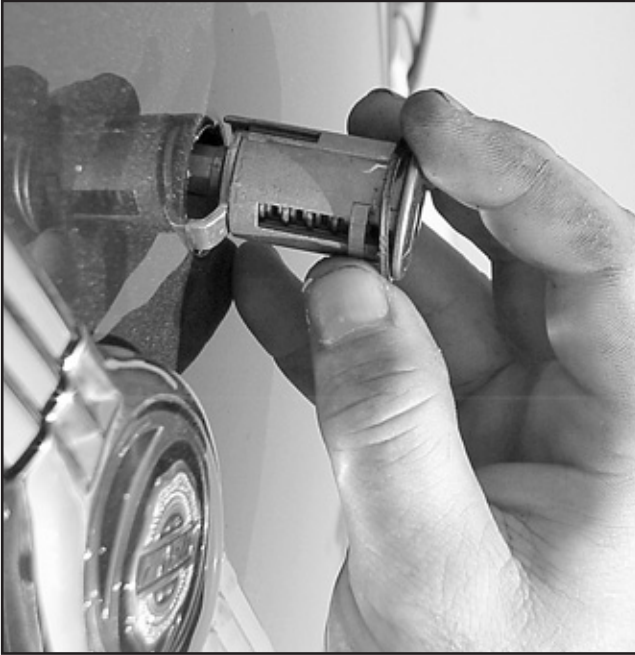
31. The lock can then be slid out the back of the tailgate.
